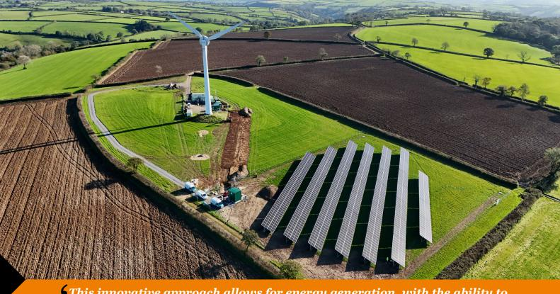
This innovative approach allows for energy generation, with the ability to balance outputs between solar and wind sources. For example, the system can flexibly allocate 200kW from solar and 700kW from wind, ensuring optimal utilisation of the 900kW maximum export capacity.
